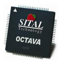
The OCTAVA<sup>™</sup> family of Mil-Std-1553 devices integrate Mil-Std-1553B protocol engine, a dual 5-volt transceiver, memory management, processor interface logic, and 4K or 64K words of RAM in a 72 Pin Plastic Quad Flat Pack (PQFP) package.
