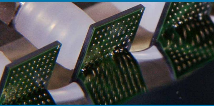
Micross is the industry-recognized leader in innovative component modification technologies, with our BGA reballing process that flushes all lead-free balls and alloy residue from pads and replaces with tin-lead balls.
