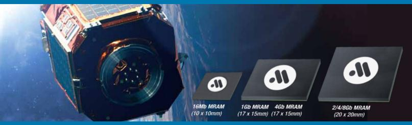
QED space-grade MRAM utilizes spin-torque transfer (STT) magneto-resistive random-access memory in a plastic BGA, qualified to NASA/Goddard Space EEE-INST-002, Level 2 PEM. STT-MRAM provides true random read/write access and inherently high resistance to magnetic flux & radiation.
