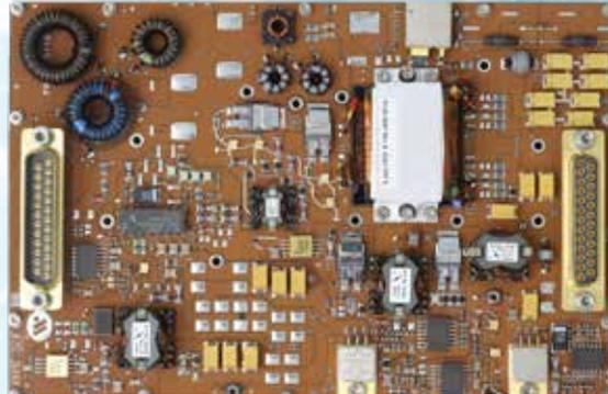
Micross' TPSU converter offers state of the art performance and is specifically designed for synthetic aperture radar applications. The TPSU provides excellent suppression of pulsed load current from output to input, and can be tailored to the specific spacecraft bus and equipment requirements.
